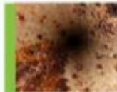
▶ EROSION Min. 10% of wall thickness
